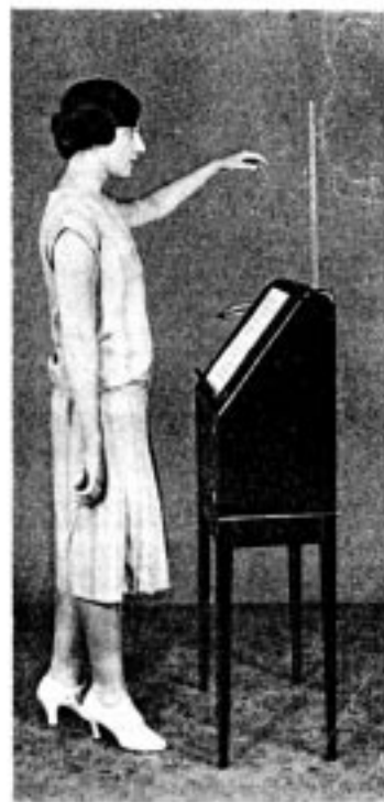
Fig. 9. Left-hand Position for Maximum Volume
